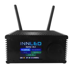
Its LCD colour screen and its rotary knob ensure easier navigation within the menu and offer a better visibility on the frequencies.
