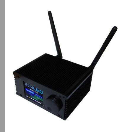
1. LCD screen with HF sniffer
