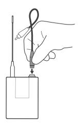
Plug the compatible adapter cable to the 3rd party trasnsmitter
